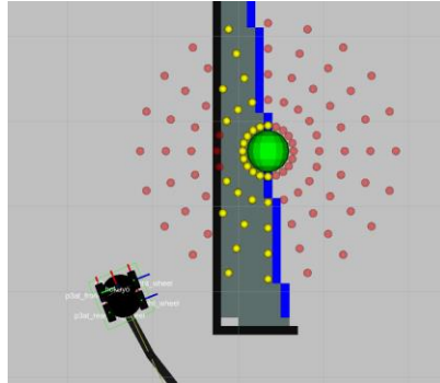
Fig. 3.5. Proposed cell sampling method. Here, the blue line indicates the chain of cells between the explored and unknown space. The green marker indicates the location of the candidate frontier p_f(x, y)_i . The red markers indicate samples that fall into the explored or occupied space. Yellow markers indicate samples located on the undiscovered cells (Semenas, Bausys & Zavadskas, 2020)
