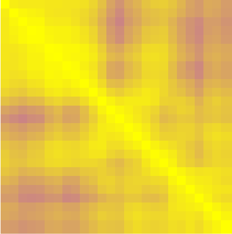
Fig. 2.4. Measure of the linear correlation of LFBE features ( |R_{i,j}| from Equation 2.1. Purple means no linear correlation, yellow means a perfect linear correlation
