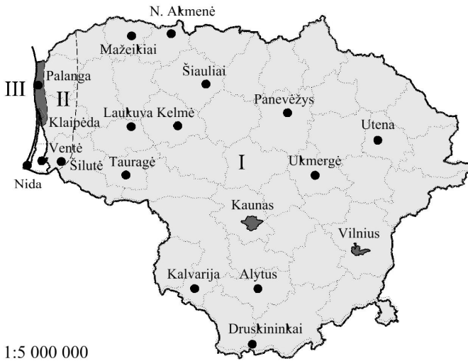
Fig. B.5. The map of basic reference wind speeds v_{ref,d} specified in the design code STR 2.05.04:2003 (see also Table B.1)
