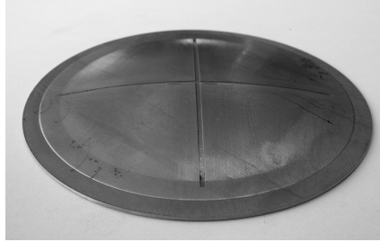
Fig 10. Diaphragm with incisions under deformation
