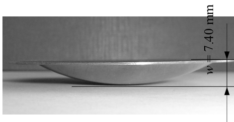
Fig 9. Shock tube diaphragm under deformation
