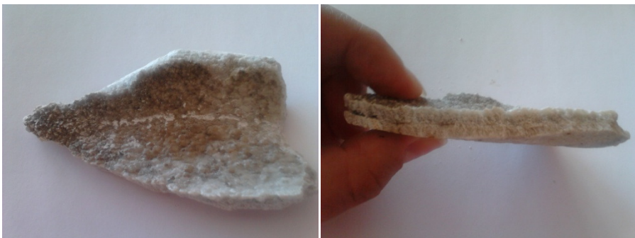
Fig. 2.1. Precipitates, formatted at Utena wastewater treatment plant
