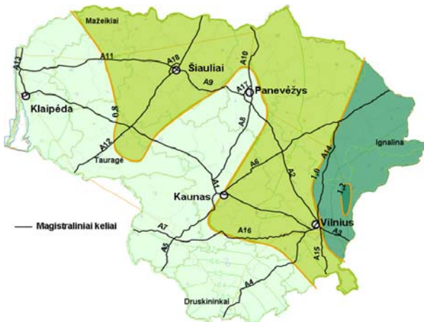
Fig. 3. Distribution of the maximum depth of frozen ground in the territory of Lithuania based on RWIS data
