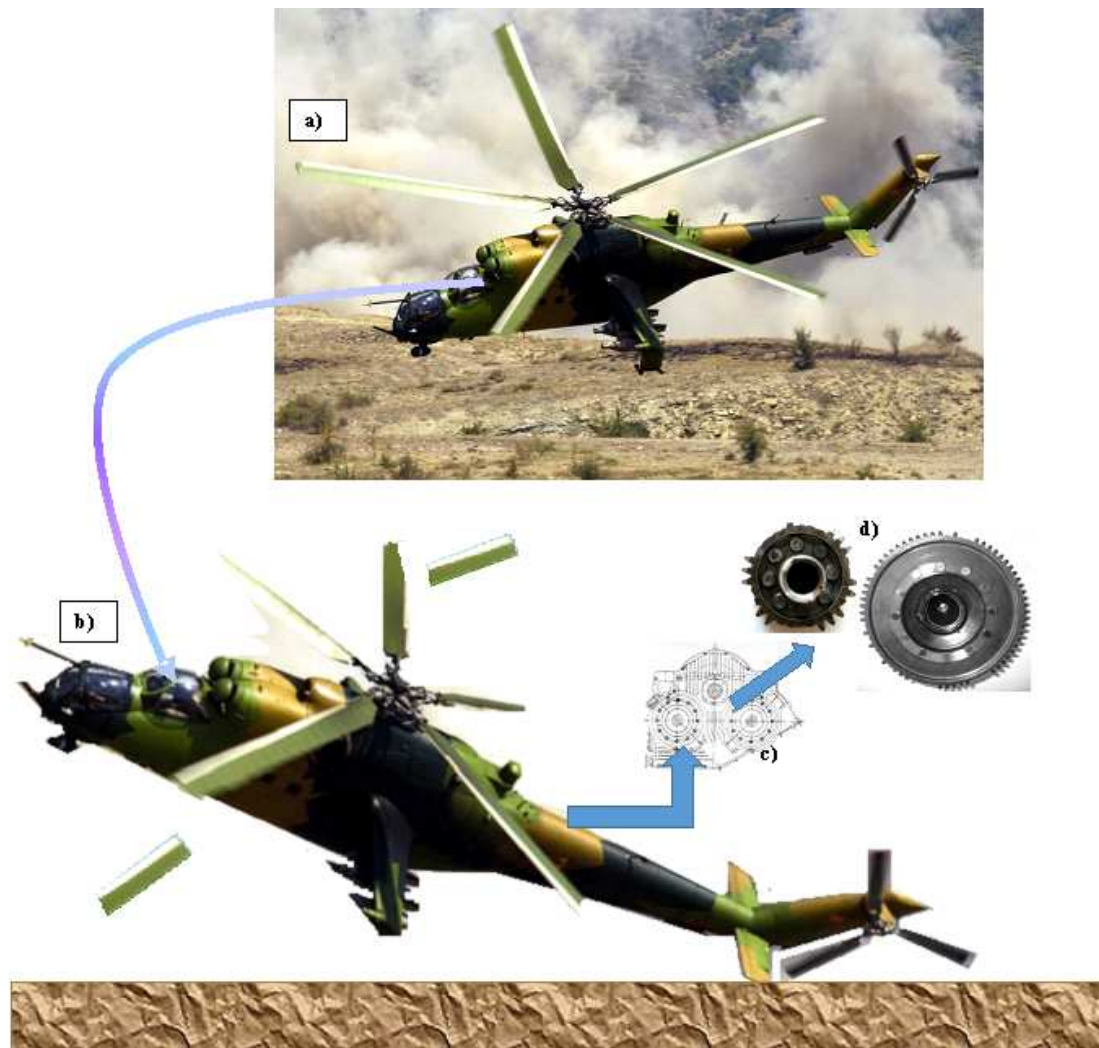
Fig. 4. The Mi-24 helicopter with a broken transmission system towards the tail rotor - due to internal damage in the generator drive box (Afghanistan 2011): a) helicopter during flight - disruption of the tail rotor drive causes it to tilt to the port side and turn left; b) the helicopter touching the aerodrome plane; c) the aggregate drive box (SNA) after breaking out of the tail beam plating; d) - broken teeth in the SNA, causing the power transmission to the rotor of the tail rotor to be interrupted
