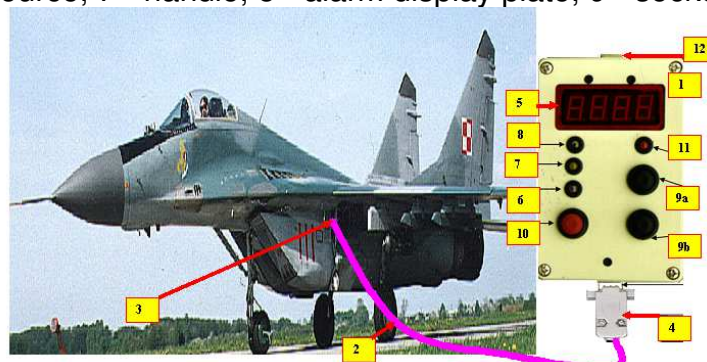
Fig. 2. Diagnostic tester DIA-KSA-CM against the MiG-29 aircraft: 1 - housing of the diagnostic tester DIA-KSA-CM; 2 - cable connecting the tester with the on-board AC power network 1x115 V, 400 Hz; 3 - electrical connector in the recess of the left landing gear; 4 - CANON DB9 connector of the tester input circuit; 5 - display; 6 - green LED diode indicating safe operation status; 7 - yellow LED indicating partial wear; 8 - red LED to indicate failure or failure status; 9 - manipulation buttons ("+" and "-") for entering the airplane number, engine designation and searching diagnostic data for a given test; 9a - manipulation button "+" (when pressed before the test, the entered tactical number of SP changes ascendingly; when pressed after the test, a symbol of a mechanical element of the power unit with a higher wear level is displayed); 9b - manipulation button "-" (when pressed before the test, the entered tactical number of SP changes decreasingly; when pressed after the test, the
