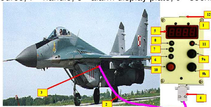
Fig. 2. Diagnostic tester DIA-KSA-CM against the MiG-29 aircraft: 1 - housing of the diagnostic tester DIA-KSA-CM; 2 - cable connecting the tester with the on-board AC power network 1x115 V, 400 Hz; 3 - electrical connector in the recess of the left landing gear; 4 - CANON DB9 connector of the tester input circuit; 5 - display; 6 - green LED diode indicating safe operation status; 7 - yellow LED indicating partial wear; 8 - red LED to indicate failure or failure status; 9 - manipulation buttons ("+" and "-") for entering the airplane number, engine designation and searching diagnostic data for a given test; 9a - manipulation button "+" (when pressed before the test, the entered tactical number of SP changes ascendingly; when pressed after the test, a symbol of a mechanical element of the power unit with a higher wear level is displayed); 9b - manipulation button "-" (when pressed before the test, the entered tactical number of SP changes decreasingly; when pressed after the test, the
