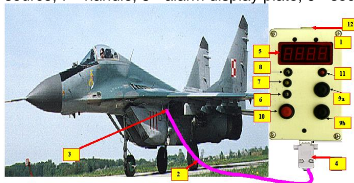
Fig. 2. Diagnostic tester DIA-KSA-CM against the MiG-29 aircraft: 1 - housing of the diagnostic tester DIA-KSA-CM; 2 - cable connecting the tester with the on-board AC power network 1x115 V, 400 Hz; 3 - electrical connector in the recess of the left landing gear; 4 - CANON DB9 connector of the tester input circuit; 5 - display; 6 - green LED diode indicating safe operation status; 7 - yellow LED indicating partial wear; 8 - red LED to indicate failure or failure status; 9 - manipulation buttons ("+" and "-") for entering the airplane number, engine designation and searching diagnostic data for a given test; 9a - manipulation button "+" (when pressed before the test, the entered tactical number of SP changes ascendingly; when pressed after the test, a symbol of a mechanical element of the power unit with a higher wear level is displayed); 9b - manipulation button "-" (when pressed before the test, the entered tactical number of SP changes decreasingly; when
