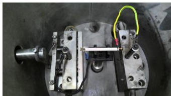
Figure 1 - Flash Joule Heating chamber.
