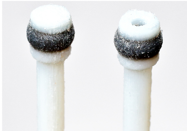
Figure 6. Three-dimensional-printed pistons integrated with the piston rod and seal [41].
