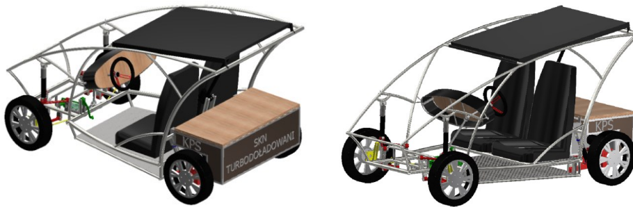
Fig. 1. CAD Model of the lightweight electric vehicle designed by the Student Research Group „Turbodoładowani” at the UTH Radom
