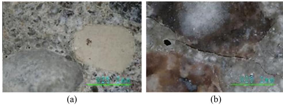
Fig. 10. Concrete structure of samples from sleepers: a – before soaking in alkali solution; b – after soaking for 46 days.
