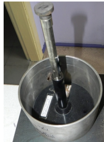
Fig. 2. Equipment for bulk density measurement (1 - metal plate, 2 - needle caliper, 3 – cylinder)
