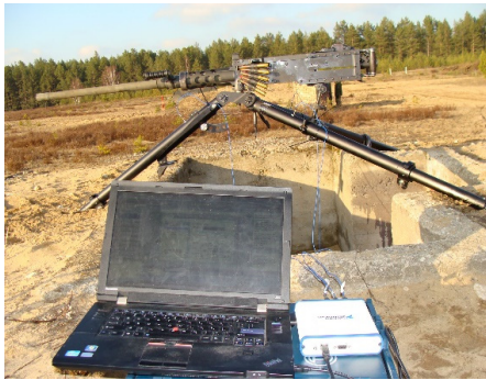
Fig. 4. Recoil force measurement equipment
