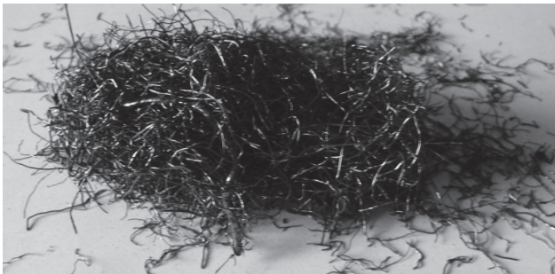
Fig. 2. Steel cord reclaimed from end-of-life tires.
