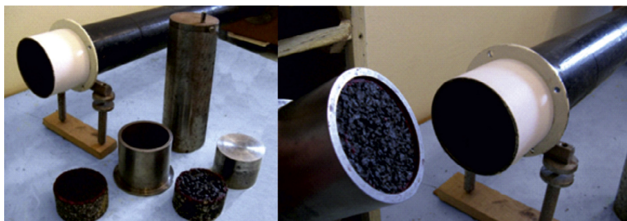
Fig. 3. Common view of 2 tested samples, sample holder, piston disk and open end of impedance tube.
