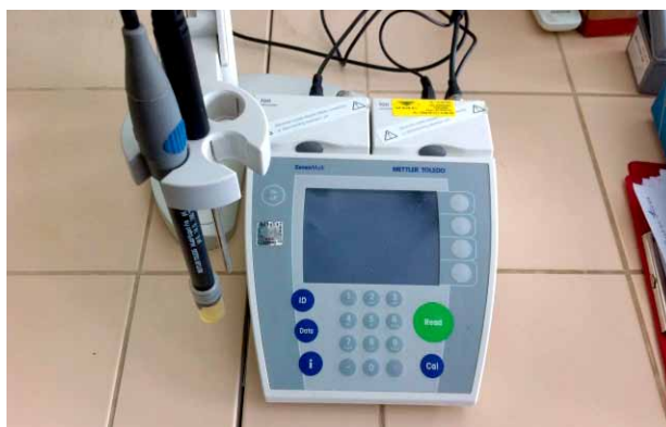
4 pav. pH-metras Metrel Toledo su stiklo elektrodu Fig. 4. pH-metter “Metrel Toledo” with glass electrode
