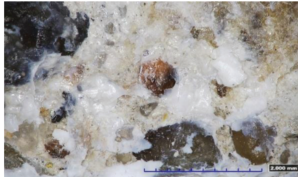
Fig.10. Traces of silica gel found with optical microscope
