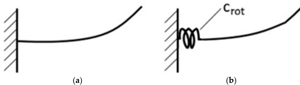
Figure 3. Type of Timoshenko beam connection to the ground: (a) fixed; and (b) through elastic spring with rotational stiffness C_{rot} .
