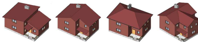
Fig. 1. Roof shapes: mono-pitched, gable and hip roof
