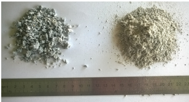
Fig. 1. Dried paper sludge (left) sieved through 2.5 mm sieve (right).
