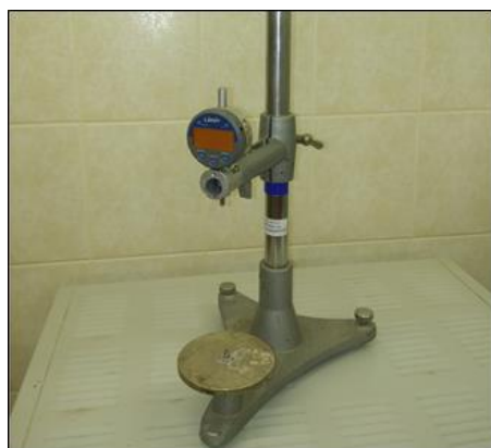
Fig. 1. Digital dial indicator and frame.
