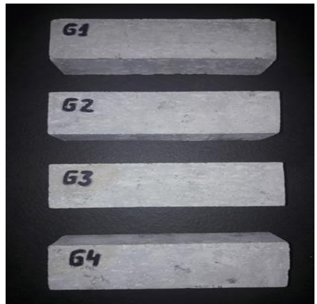
Fig. 9. Photos of specimens with granite rubble fr. 5/11 (Mix G) after 56 days soaking in 1 M NaOH solution.
