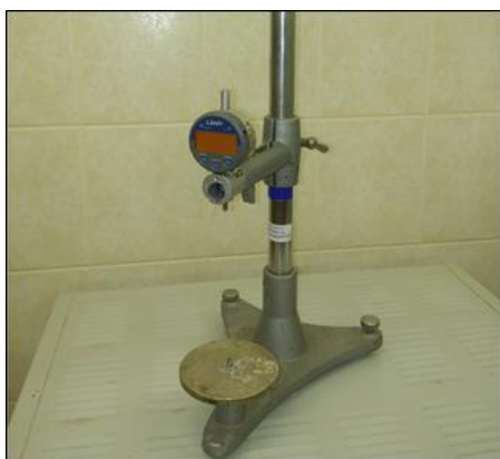
Fig. 1. Digital dial indicator and frame.
