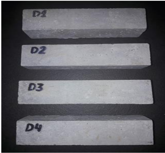
Fig. 5. Photos of specimens with granite rubble fr. 2/8 (Mix D) after 56 days in 1 M NaOH solution.
