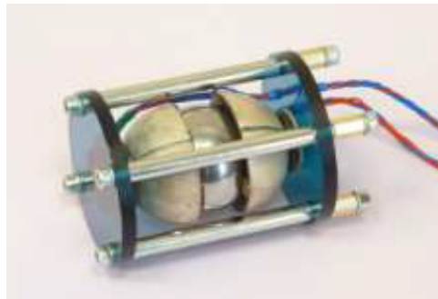
Fig. 6. Test example of sphere with two hemispheric piezoelectric transducers
