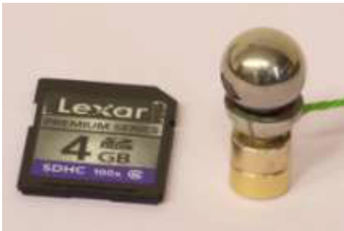
Fig. 5. Laboratory test example of sphere with implementation of permanent magnet for sphere attachment
