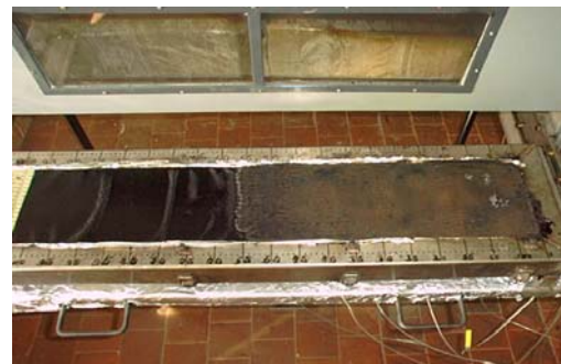
Fig. 6. The image of Fragment System 1.1 after the burning test
