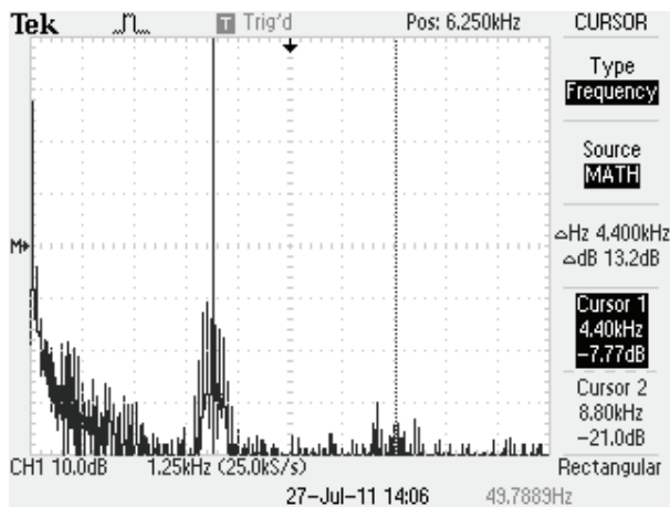
Fig.6. The attenuation of the carrier signal first harmonic by the L-C-R filter of the inverter when carrier frequency is 4.4 kHz and capacitance of filter capacitor is 6.8 \mu\text{F}
