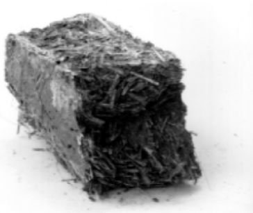
Fig 9. Fractured composite specimen containing 70 % of aluminate cement 40, 20 % of boon and 10 % of CMC (dry solids)
