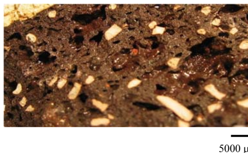
Fig. 8. Picture of the sample with non-milled catalyst after burning at 1150 °C temperature
