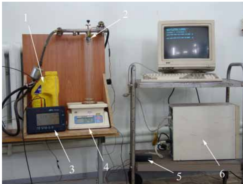
Fig.1. Stand for measuring the amount of the ejected ethanol: 1 – fuel tank; 2 – electromagnetic nozzle for ethanol; 3 – temperature gauge; 4 – electronic scales; 5 – impulse generator, 6 – PC
