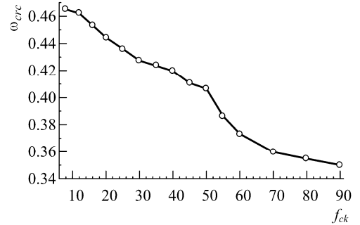
Fig. 2 Relation between relative coordinate of the centroid \omega_{crv} and characteristic strength of the concrete
