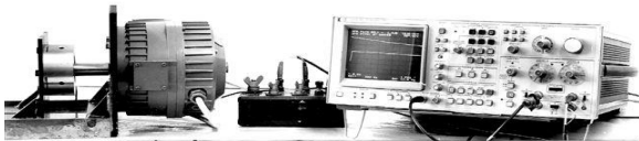
Fig. 4 Test rig to calibrate a Ferraris sensor
