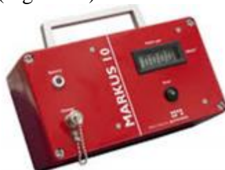
Figure 4 Markus 10 type instrument for measuring radon level
