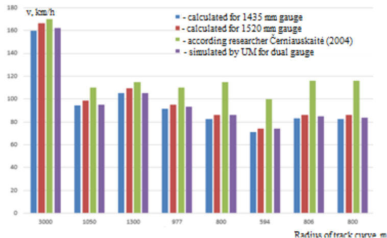
Fig. 6. Comparison of the research results and the calculated maximum speed on „Rail Baltica“ track curves
