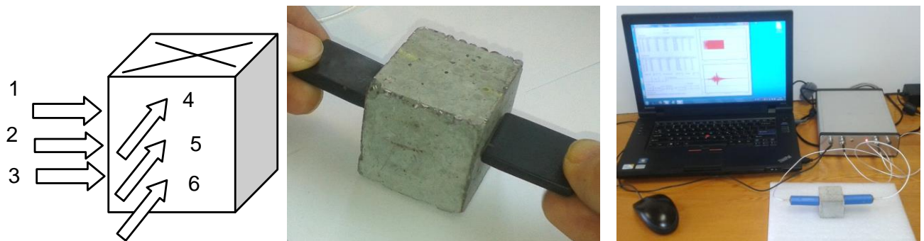
Fig. 1. Illustrations of US testing: directions of through transmission (left); application of transducers (middle) and acquisition setup (right).
