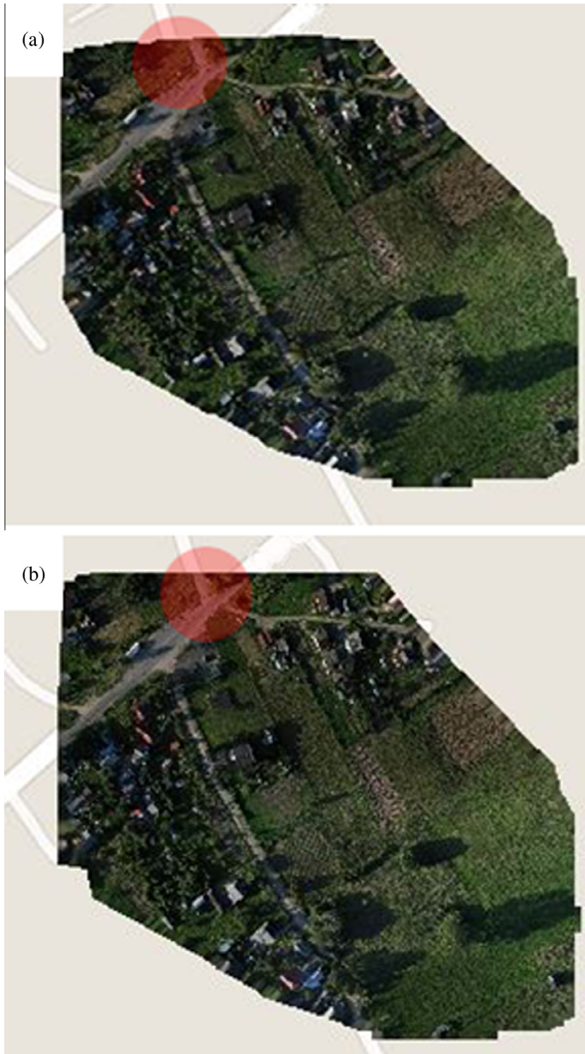
Fig. 4. Generated orthophoto with vector data overlaid (red dot shows fragment of situation for comparative analysis): (a) images rectification using PCC, (b) applying 10 GCPs. (For interpretation of the references to colour in this figure legend, the reader is referred to the web version of this article.)
