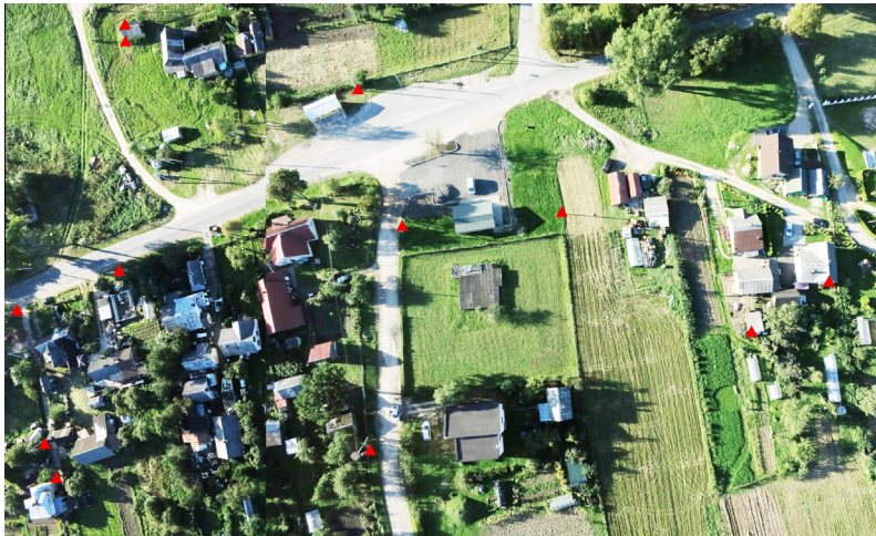
Fig. 3. Distribution of ground control points (marked by red triangles) on the test area. (For interpretation of the references to colour in this figure legend, the reader is referred to the web version of this article.)
