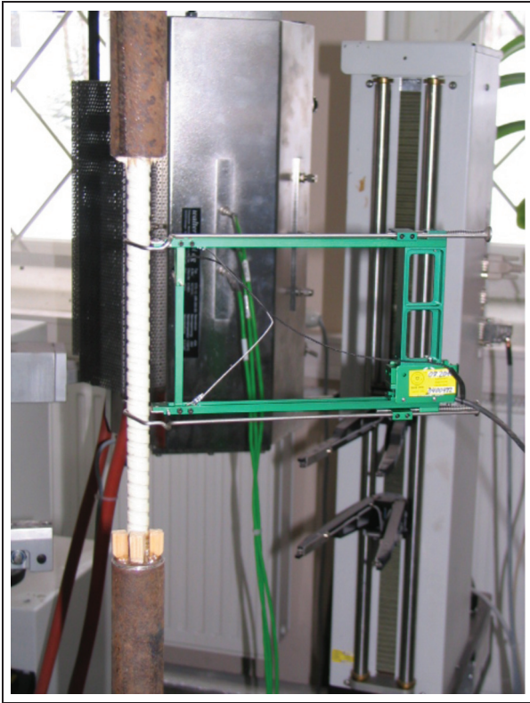
Figure 3. Testing of the GFRP reinforcement bar.
