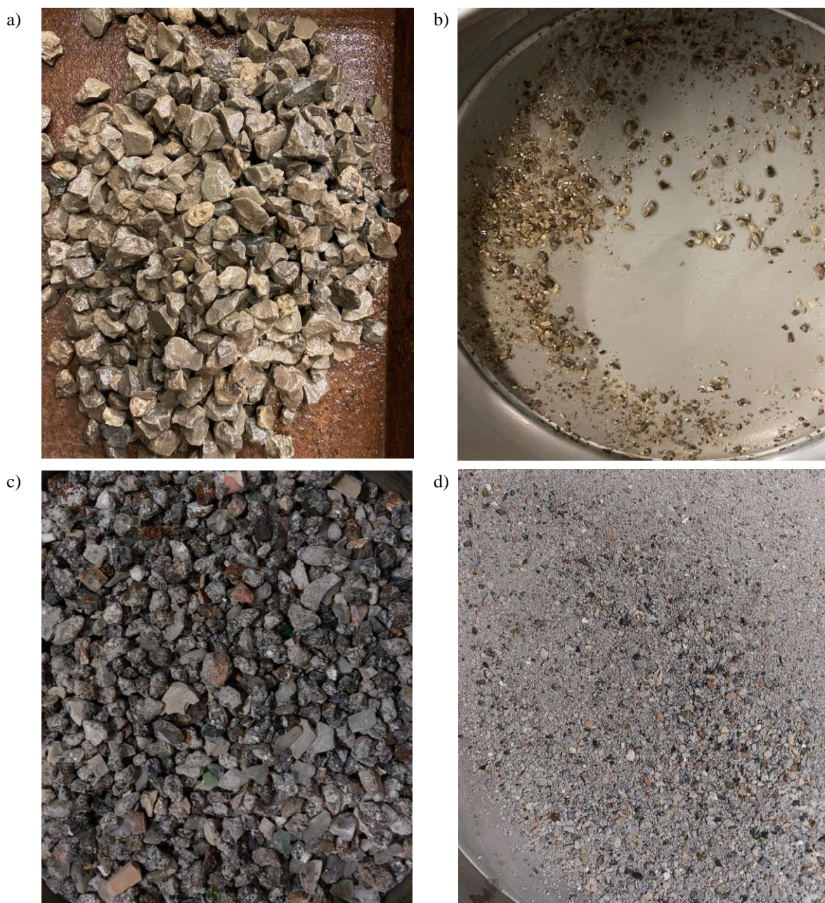
Figure 2. Retained aggregate on the 4 mm sieve and that passed through 0.063 mm sieve after 10 freeze-thaw cycles: a, b) reference aggregate (crushed dolomite); c, d) MSWI bottom ash
