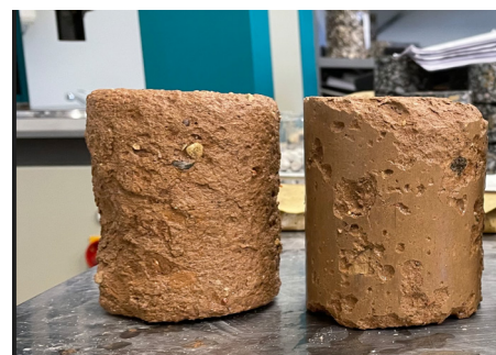
Figure 6. Treated clay specimens after freezing cycles before compressive strength test (3% of cement with 0.15 L/m 3 Stabgrunt 1 – on the left; 5% of cement with 0.15 L/m 3 Stabgrunt 1 – on the right)
