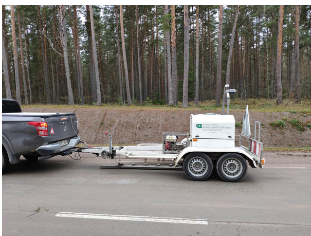
Figure 4. Testing device – falling weight deflectometer (FWD)
