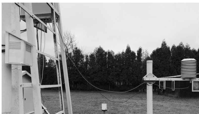
Fig. 6. Device prototype (on the left) mounted at same height sensor (on the right) – reference station Rogow (Fig. P. Szymanski)
