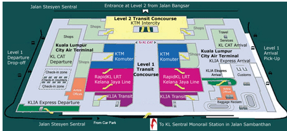
Fig. 1. Kuala Lumpur Sentral layout Transit Concourse, Level 1 : Urban public transit services such as the KTM Komuter, KLIA Transit and the Kelana Jaya Line light rail transit. Transit Concourse, Level 2 : KTM intercity trains. KL City Air Terminal (KLCAT): KLIA Ekspres, and the high-speed rail service to Kuala Lumpur International Airport (KLIA). (KL Sentral Station 2016)
