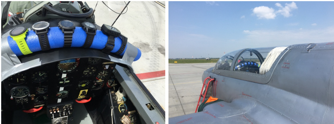
Fig. 3. Installation of GNSS equipment during the test flight. From the left: Suunto Ambit 3, Garmin D2 Bravo, Garmin Fenix 3, Garmin Fenix 2, Garmin Foretrex 401, Garmin Forerunner 610
