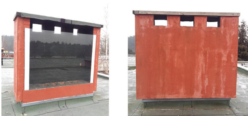
Fig. 2. The tested solar chimney
