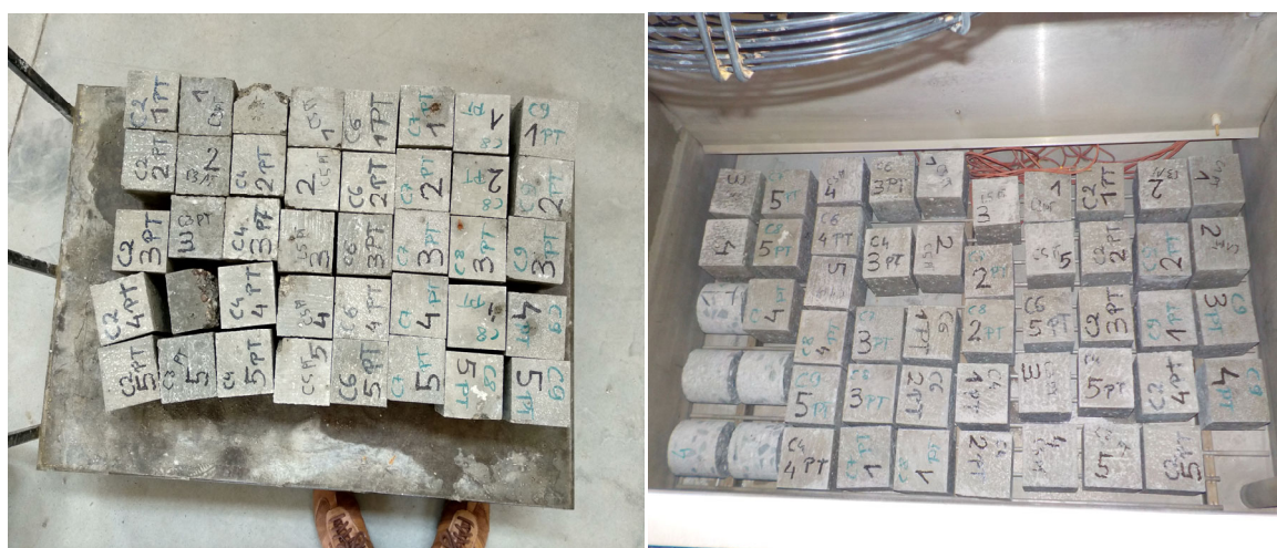
Figure 1. Specimens before and after 150 freeze/thaw cycles
