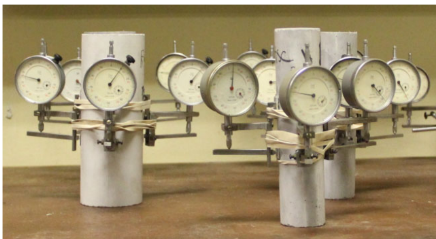
Figure 2. Prepared samples for shrinkage and creep tests
