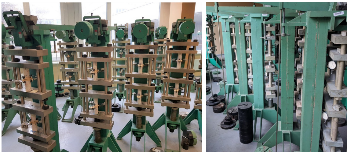
Figure 3. Specimens on creep test lever stands
