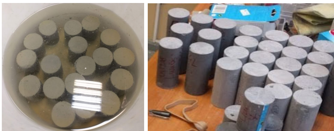
Figure 4. Water saturated and air-dry foam concrete specimens
