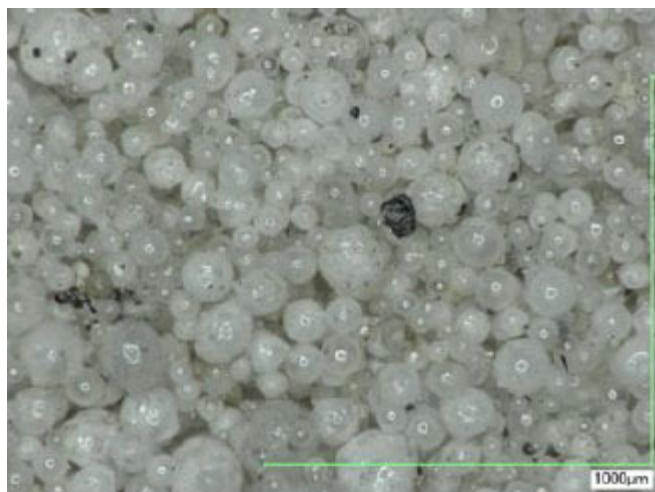
Figure 1. Porous aggregate used in the mixes of FC (microscope image of CS)
