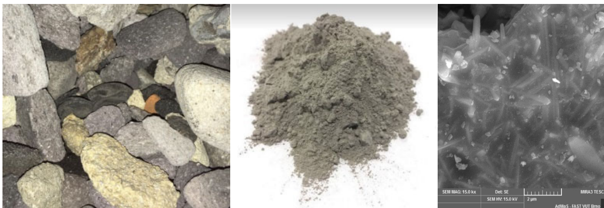
Figure 1. In the left images – unmodified fireclay waste, In the middle images – fireclay waste after adjusting the specific surface to 253 m 2 /kg, In the right images – SEM image of fireclay waste
