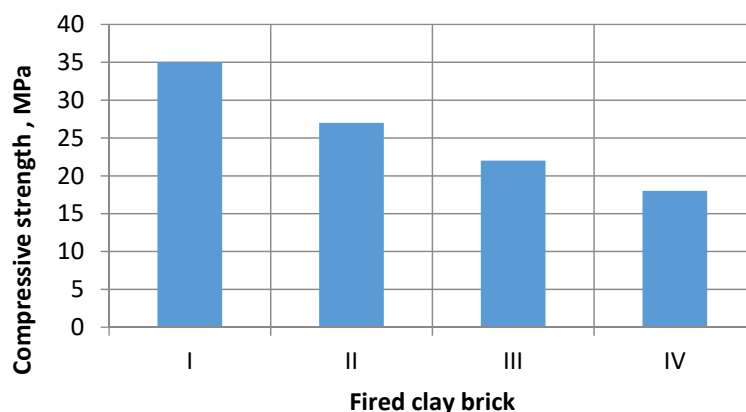
Figure 5. Compressive strength of fired clay brick
